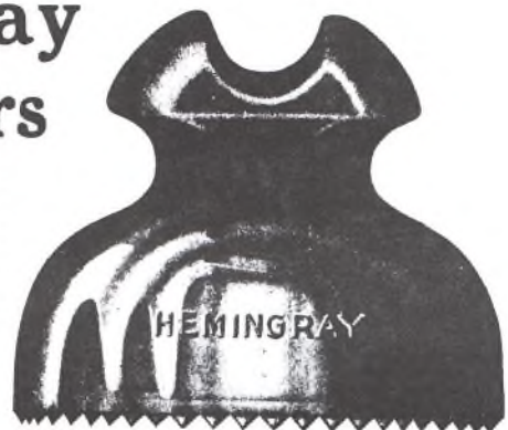
No. 72—Voltages—Test—Dry 64000, Wet 31400, Line 10000
